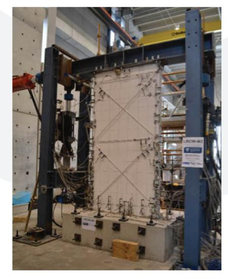
The behaviour of six phase I test walls designed in accordance
