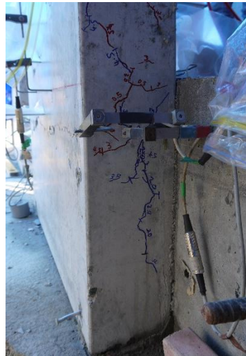
Figure 6: Joint condition of a conventional starter bar connection (Panel U12-C50)
