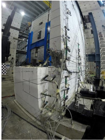
(a) Damage state at end of in-plane loading
