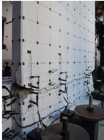
(b) Damage state at end of bi-axial loading
