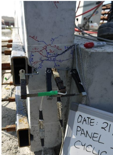
Figure 3: Damage of Panel BLT12-C0 at 4.5% drift in the joint-opening direction
