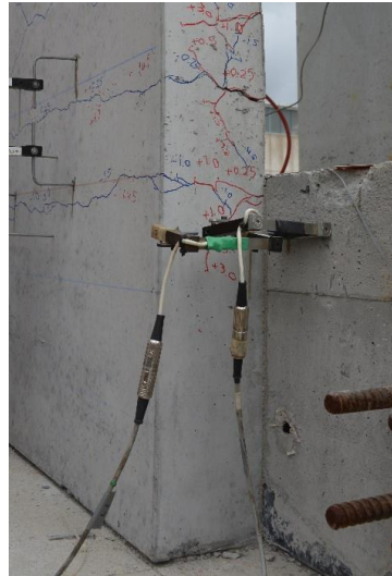
Figure 18: Joint condition of a threaded insert connection with confined joint region (Panel T112-C15-STRP)
