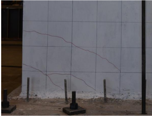
(a) Cracks resulted from threaded insert
