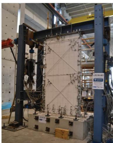
The behaviour of six phase I test walls designed in accordance with NZS 3101:2006 (A2) was controlled by 1-3 large flexural cracks at the wall base. The experimental results confirmed that current minimum vertical reinforcing limits in NZS 3101:2006 (A2) are insufficient to ensure that a large number of secondary cracks form and are only suitable for walls designed for low ductility demands.
