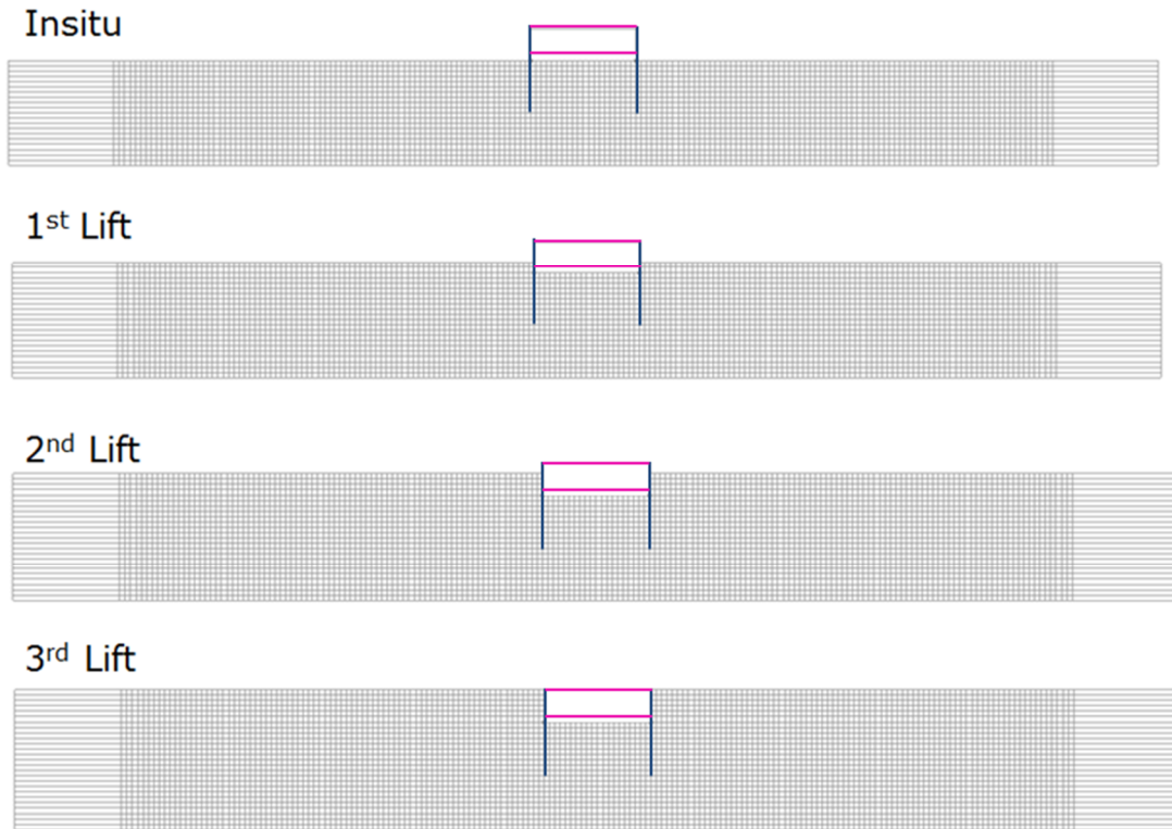
Figure 3-1: Class C Propped Wall Staged Construction
