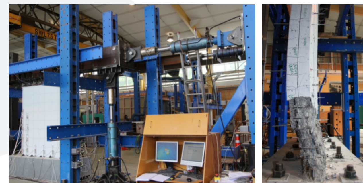
Fig 5: Test setup and out-of-plane instability of one of the specimens
