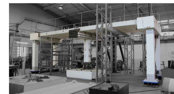
Fig 8: 1/3 scale bridge test specimen
