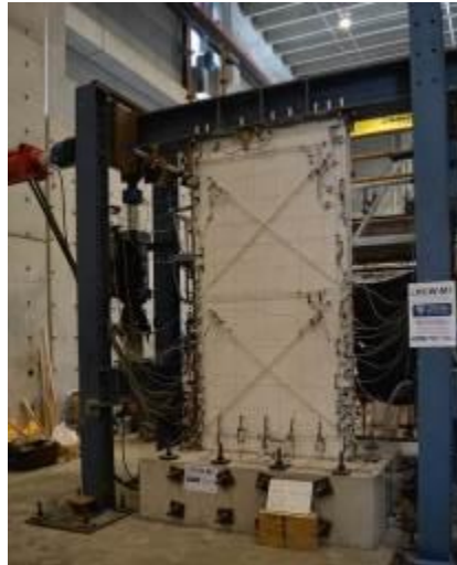
Figure 2 - Test setup and moment distribution over the wall height
