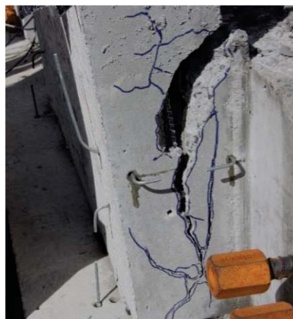
Figure 2 - Panel vertical crack propagation
