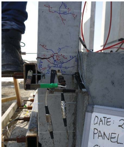
(a) Panel cracking
