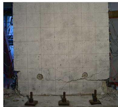
(b) Extent of flexural cracking
