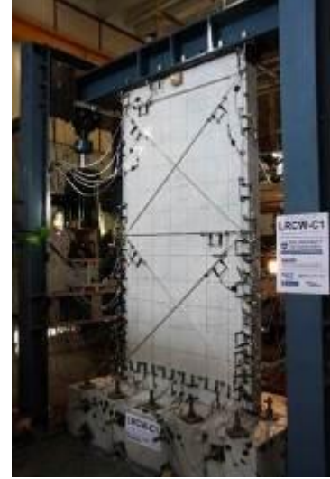
Fig. 6. Experimental test setup for RC walls
