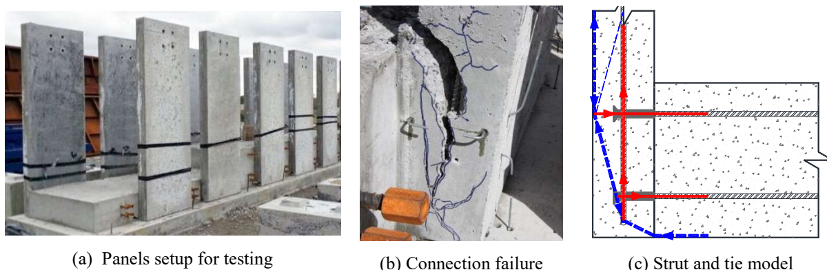
Figure 6 Out-of-plane tests of threaded insert connections
