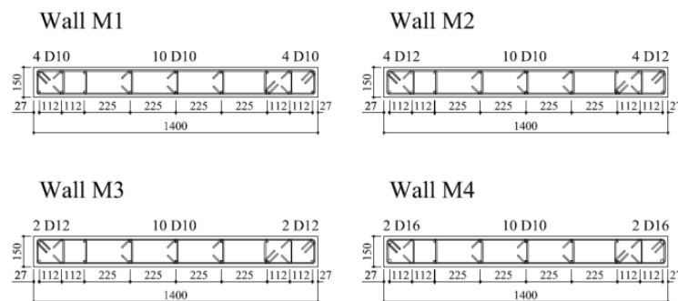
Figure 5. Cross sections of test wall specimens
