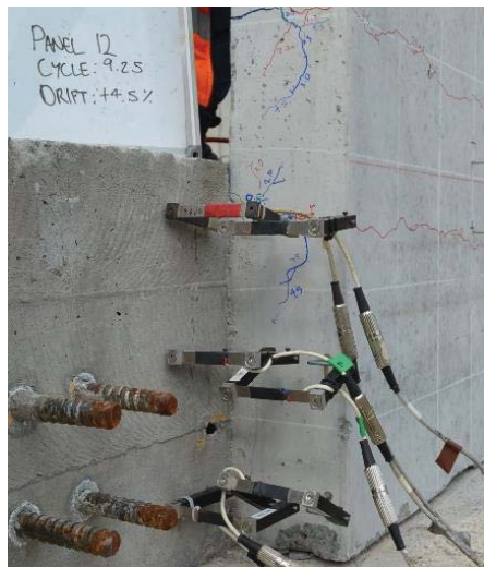
(a) Panel cracking
