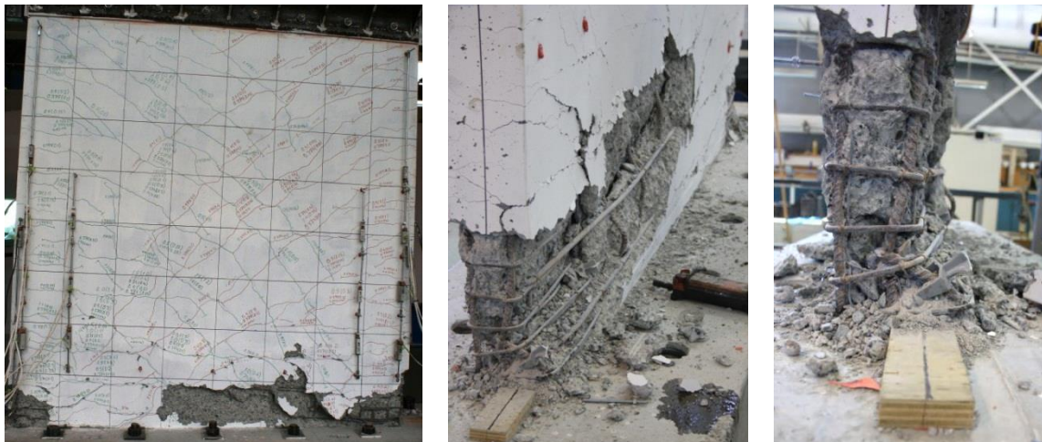
Figure 11. Instability of Specimen RWT.
