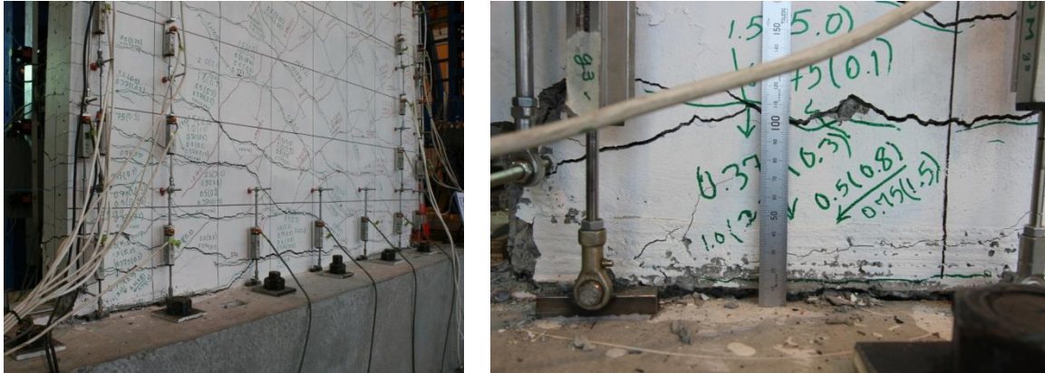
Figure 9. Wide cracks at +2.0% drift level – Specimen RWT.
