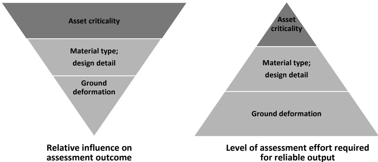
**Figure 3: Schematic presenting typical influence of resilience assessment inputs on output of assessment, and uncertainty associated with various elements.**
